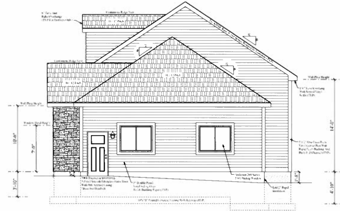
RIGHT/EAST ELEVATION SCALE: 1/4" = 1'-0"
