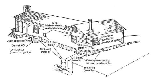
**Note 1:** Relief valve, filling connection, and liquid fixed maximum level gauge vent connection at the container must be at least 10 feet from any exterior source of ignition, openings into direct-vent appliances, or mechanical ventilation air intakes. Refer to 6.3.2
