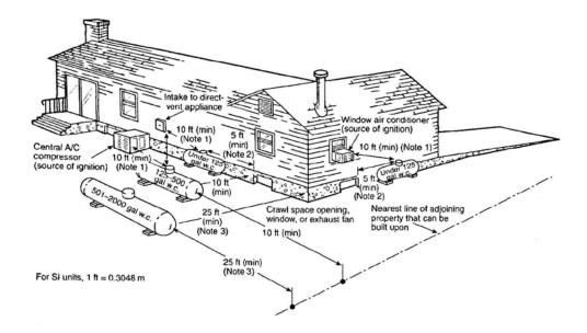
**Note 1:** Regardless of its size, any ASME container filled on site must be located so that the filling connection and fixed maximum liquid level gauge are at least 10 feet from any external source of ignition (e.g., open flame, window A/C, and compressor), intake to direct-vented gas appliance, or intake to a mechanical ventilation system. Refer to 6.3.9
